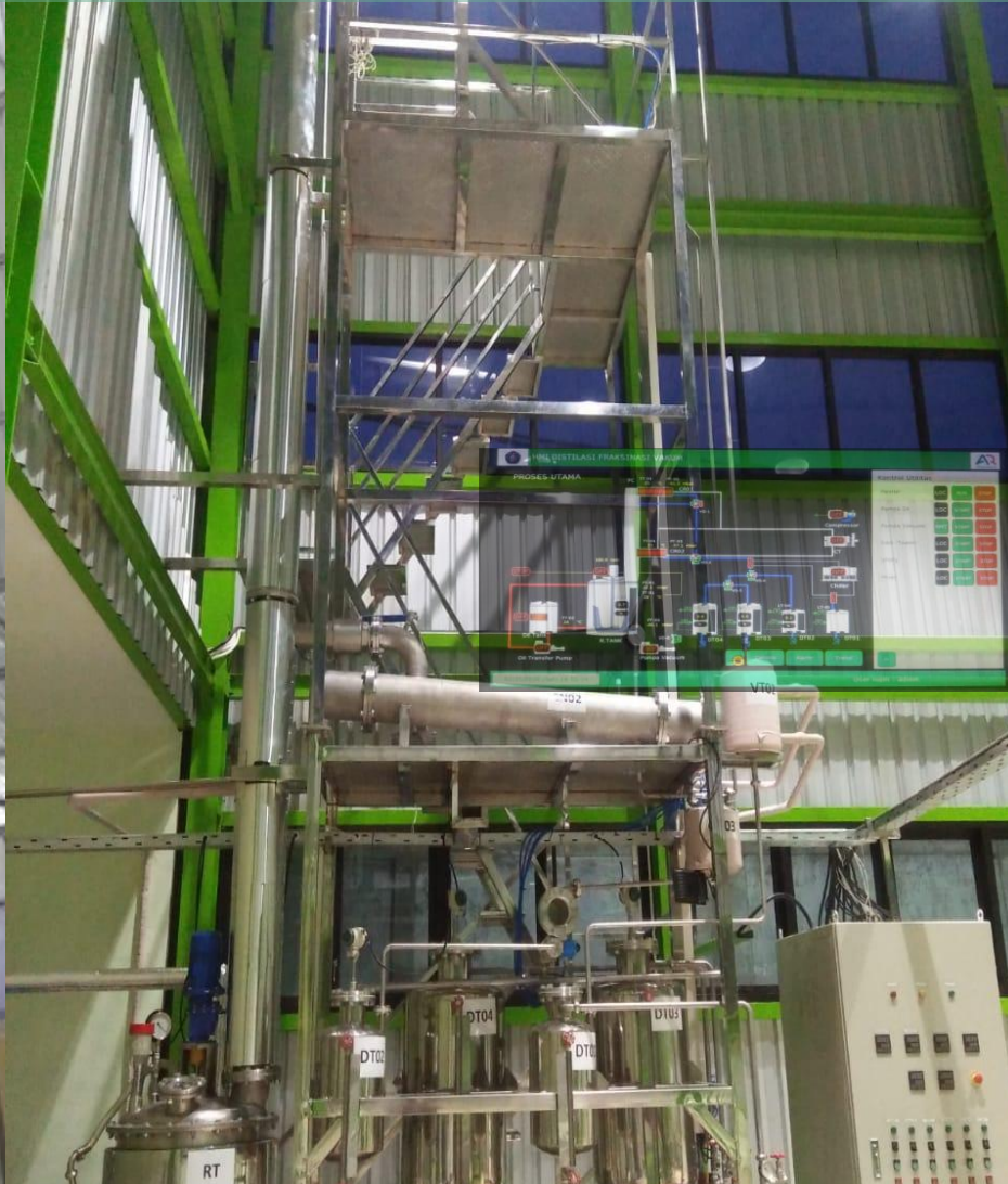
Fractionational Distillation Institut Atsiri – Universitas Brawijaya Capacity 200 lt/batch for Citronellal 80%
