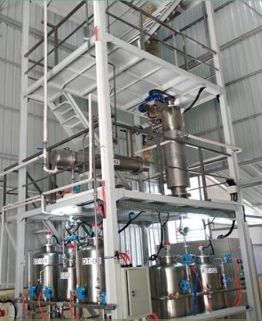
Wiped Film Fractionation Atsiri Research Center - UNSYIAH Capacity 200 lt/batch for Patchouly Oil MD
